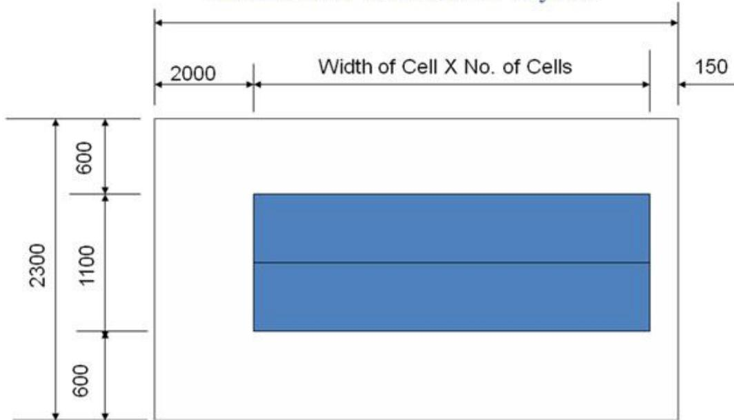
The floor of the battery room should be preferably acid resistant and no inflammable materials are to be used inside the battery room. The room should be well ventilated either by two open windows or by using suitable exhaust fan to enable continuous change of air inside the room.
